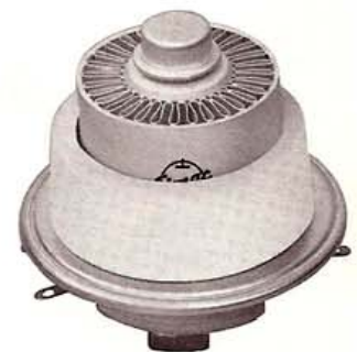
SOCKET, TUBE, AND CHIMNEY
